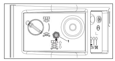
Figure 4-8. Lowering Platform From Ground Control
