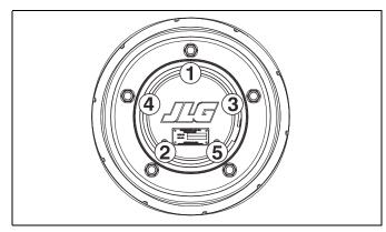
Figure 6-3. Wheel Lug Nut Tightening Sequence
