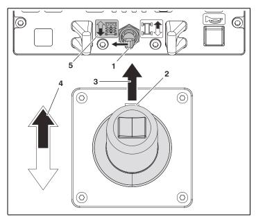
Figure 4-9. Lowering Platform From Platform Control
