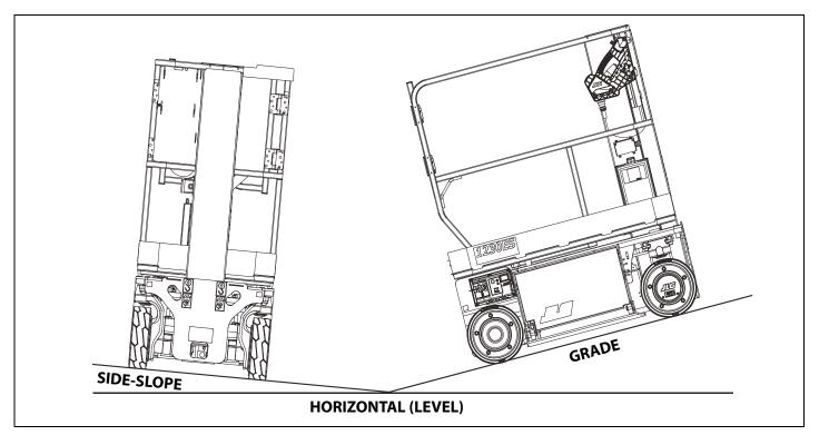
Figure 4-12. Grade and Side-Slope Definition
