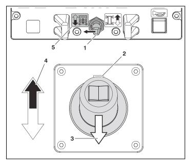
Figure 4-7. Raising Platform From Platform Control
