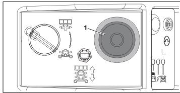
Figure 4-4. Ground Control - Emergency Stop Switch
