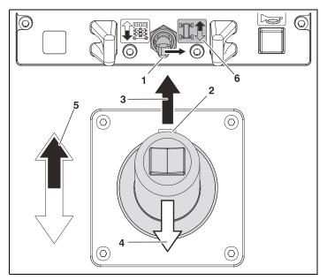
Figure 4-11. Driving Forward from Platform Control
