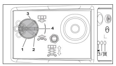
Figure 4-3. Platform/Ground Select Switch
