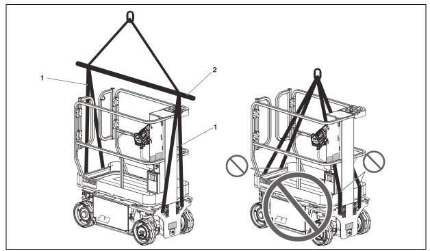
Figure 4-16. Lifting Using Spreader Bar.
