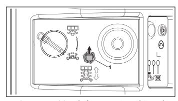
Figure 4-6. Raising Platform From Ground Control
