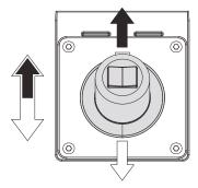
**Drive** - The drive function must be selected using the drive/lift selector switch (*items 5 and 6 on the Platform Control/Indicator panel - Figure 3-8.*), prior to moving the control handle. After selecting the drive function, engage the trigger switch lever, then move the control handle forward to drive the machine forward or move the control handle backwards to drive the machine backward.
