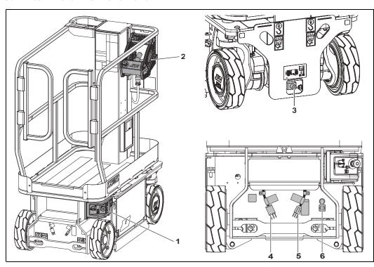
Figure 3-1. Location of Machine Controls.
