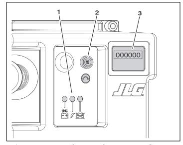
Figure 3-4. Battery Charger and Hour Meter Indicators
