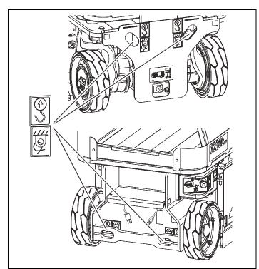
Figure 4-14. Tie Down and Lift Lug Locations.
