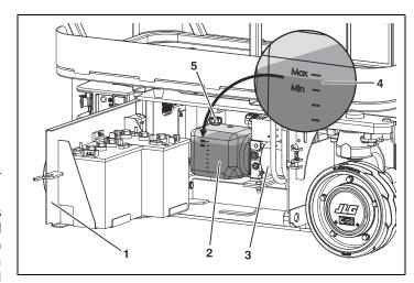
Figure 6-1. Hydraulic Oil Check Procedure
