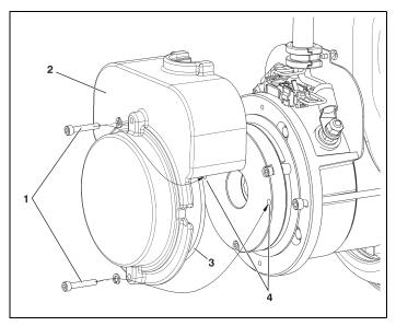
Figure 4-18. Brake - Manual Disengage.
