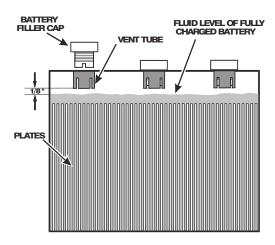
Figure 6-2. Battery Fluid Level.
